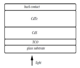
Fig (5): Basic structure of CdTe solar cell [81]
