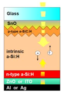
Fig (3): structure of a-Si solar cell [16].
