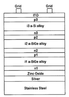
Fig (2): Triple junction structure a-Si solar cell [11]
