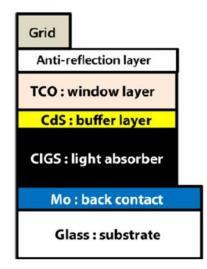
Fig (4): simple structure of CIGS solar cell [48]
