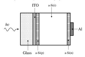
Fig (1): First structure of a-Si solar cell [7].
